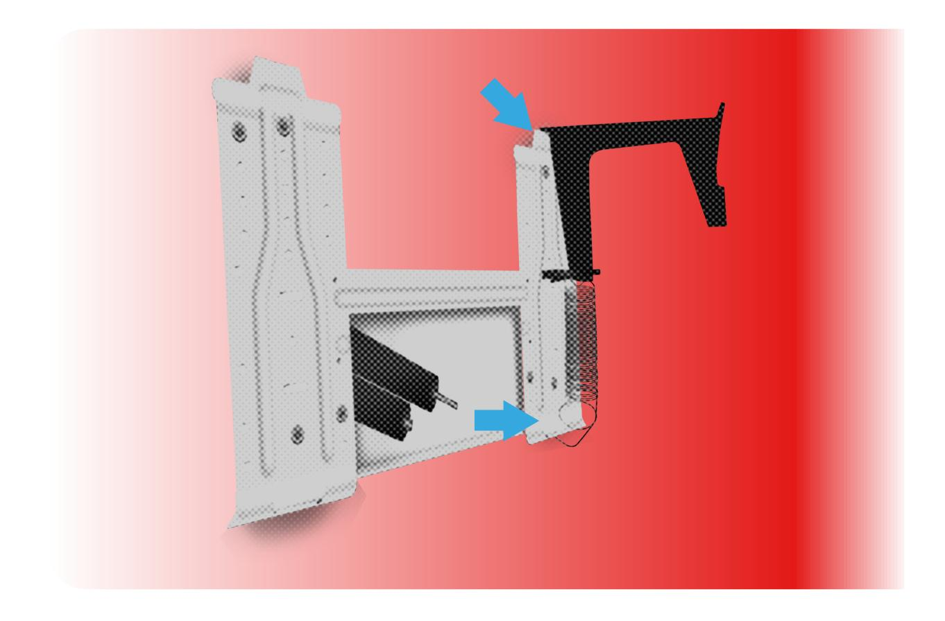
Place the SMALL bracket in the superior RIGHT hook of the plate (from viewer's position), and secure the spring on the bottom hook of the plate.
