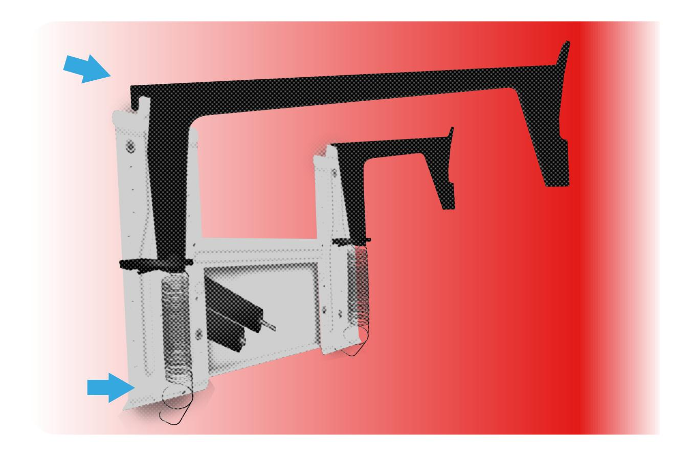
Place the LARGE bracket in the superior LEFT hook of the plate (from viewer's position), and secure the spring on the bottom hook of the plate.
